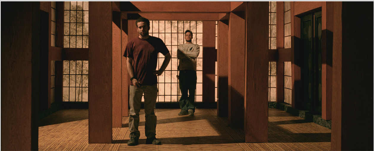
Japanese Shrine: Built on stage, this set was constructed with paper walls to incorporate a bamboo shadow effect. The bamboo floor and stone base are both faux finishes. My original CAD footprint is shown at the right.
